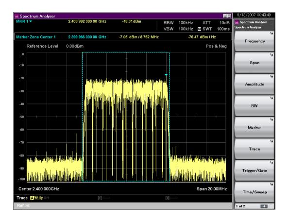
F. For Signal Analyzer functions: Select Application Switch, then Signal Analyzer (F2), Frequency (F1), Amplitude (F2), Trace (F5), and Trace Mode (F1); this will access spectrum, power vs.. time, frequency vs. time, and CCDF measurement functions.
