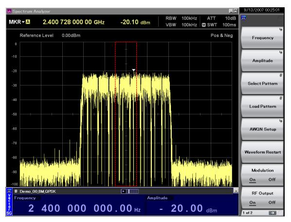
E. To view the waveform with the Spectrum Analyzer: select Application Switch and Spectrum Analyzer (F1), Setting Frequency (F1), Span (F2), and Amplitude (F3), along with other standard Spectrum Analyzer settings. It can also be set with a USB mouse or key board, if desired.
